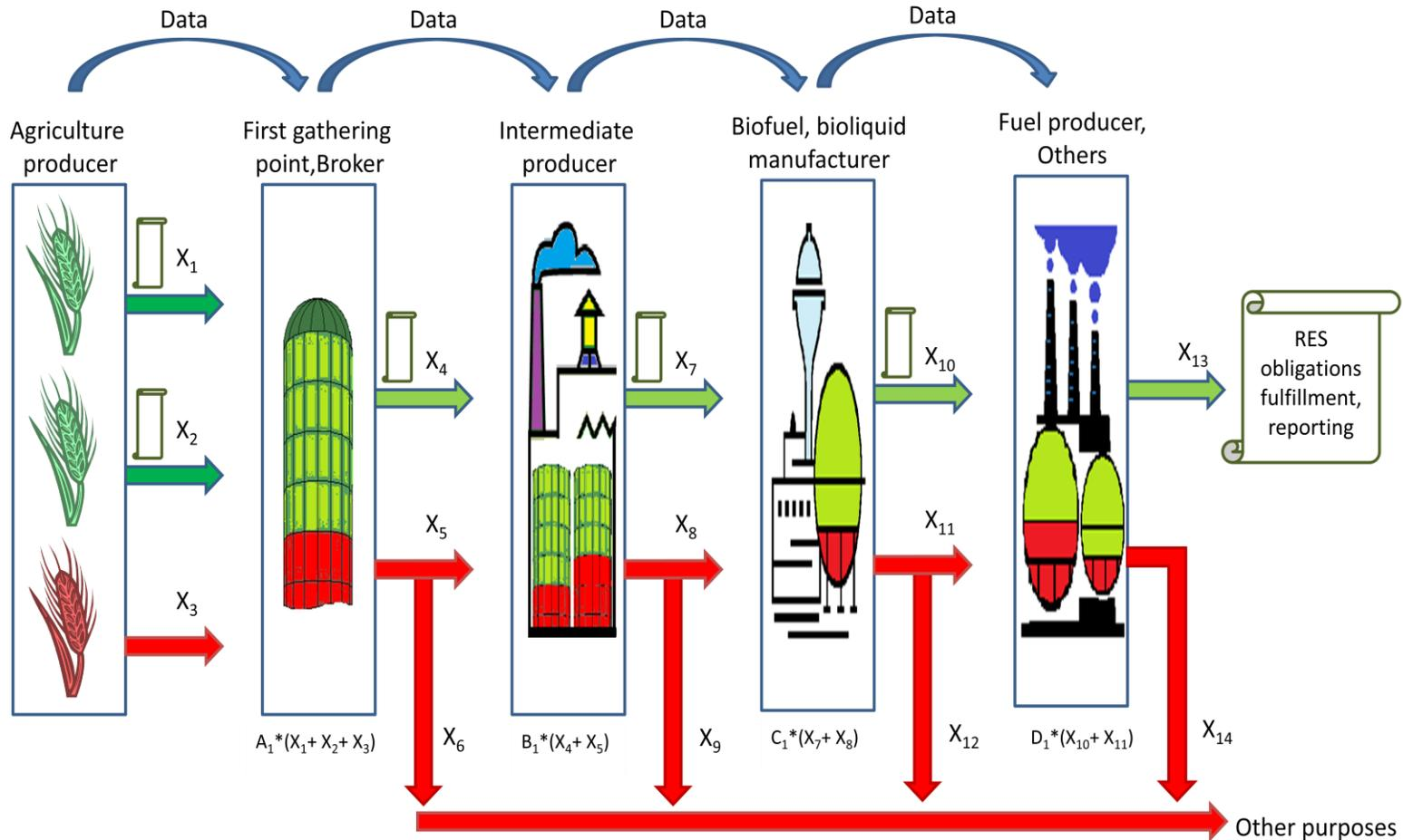
**Fig. 2 Diagram of a mass balance under the INiG System – solid biomass fuels**
